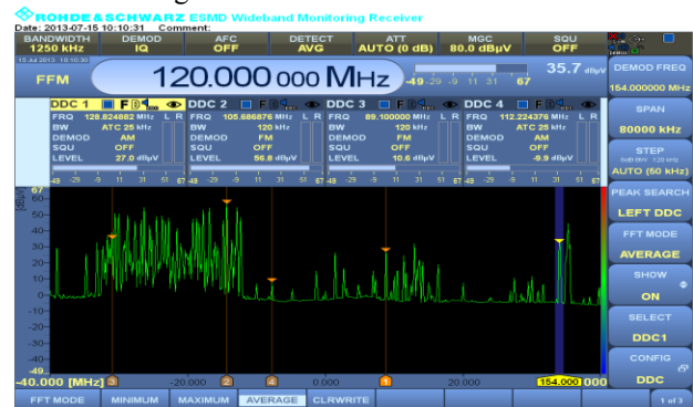
Fig. 2: Five channel arrangement for signal analysis
